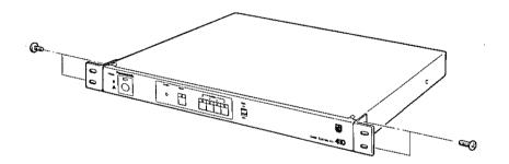
4. Install the Quad Unit WJ-410 on the EIA 19-inch rack by using four screws (Locally procured).
