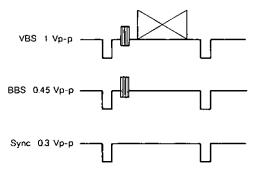
10. Sync. Output Connector (SYNC OUT) A 4Vp-p/75 ohms of composite Sync. signal is obtained at this connector in order to synchronize other cameras or a camera drive unit such as WV-PS11A, WV-PS104B etc.
